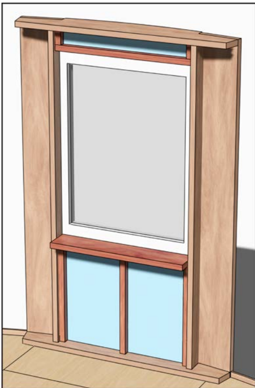
Sill and insulation
